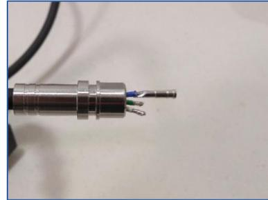
8. When all three Electrical Sockets are soldered to the wires, gently press them into the PEEK Insert by hand. Use a multimeter to make sure there are no electrical shorts between the Electrical Sockets and the Connector Shell. Note that there *will* be an electrical short from one Electrical Socket to another Electrical Socket since they are now connected to the windings in the thruster motor.
