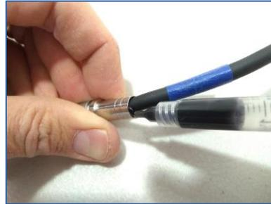
14. Push the cable jacket back all the way back into the Connector Shell. A large amount of epoxy or urethane should come out the rear of the Connector Shell, ensuring that the inside of the Connector Shell is completely filled. Clean off the excess epoxy or urethane with a paper towel and acetone or alcohol.
