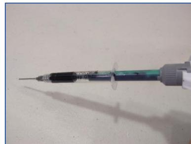
13. With the cable jacket pulled out of the Connector Shell, inject the epoxy or urethane into the Connector Shell until the epoxy or urethane starts to come out the rear of the Connector Shell. Move the cable around inside the Connector Shell to ensure that both the outer surface of the cable jacket and the inner surface of the Connector Shell are fully wetted with epoxy or urethane.
