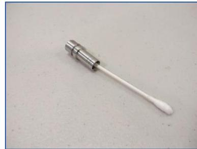
3. Slide the Locking Sleeve onto the thruster cable with the internally threaded part of the Locking Sleeve facing towards the end of the cable. Place a piece of tape on the cable to keep the Locking Sleeve from coming off.
