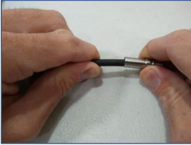
11. Put a piece of tape on the cable jacket immediately adjacent to the Connector Shell. Now pull the cable jacket back out of the Connector Shell. There should be at least 15 mm of cable jacket beyond the tape. If there is less than 15 mm of cable jacket beyond the tape, repeat the previous step.
