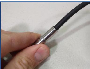
16. Lubricate the O-ring and install it in the groove on the Connector Shell, making sure that the groove and the O-ring are free from lint, hair, or other contamination.
