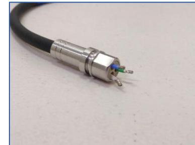
7. Tin the wires with solder. Then place an Electrical Socket on each wire and solder it to the wire. It is very important that the solder remains inside the solder cup on the Electrical Socket. If solder gets on the outside of the Electrical Socket, it may make it impossible to press the Electrical Socket into the PEEK Insert.
