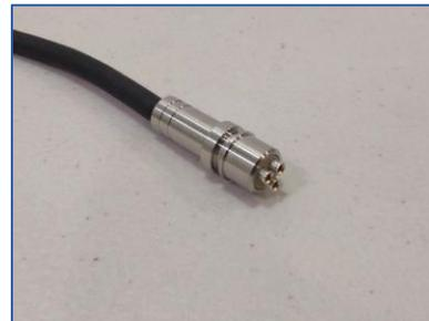
9. Gently hold the Connector Shell vertically in a vise. Mount the Dowel Pin in a drill press chuck and use it to carefully press each Electrical Socket into the PEEK Insert. Go slowly and be careful: once the Electrical Sockets are pressed in, they cannot be removed. Use the multimeter to check again for electrical shorts between the Electrical Sockets and the Connector Shell.
