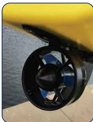
Powerful differential thrusters for maneuverability
